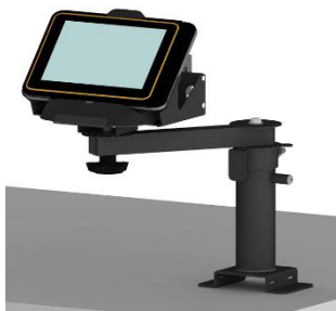
PN 80080-505 - Countertop Fixed Pedestal Mount with a 6" riser, adjustable 8" arm + panning head for a MICROS 720 Tablet with drop in charger
