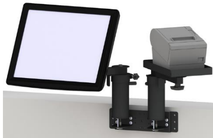
PN 80026 - Wall Mount with two 6 inch Risers, two 8 inch Arms, a 75/100mm VESA Screen Pan and Tilt Head, & a Flat Printer Tray
